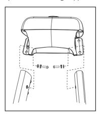
Figure 8: Rear view of console attachment
