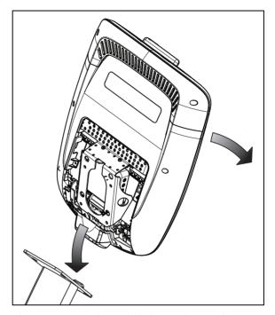
Figure 23: Console positioning on base unit
