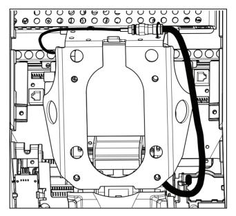
Figure 25: Connecting the television cable
