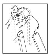
Figure 9: Center column support attachment
