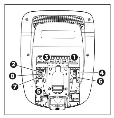
Figure 24: Cable connections, P80 console
