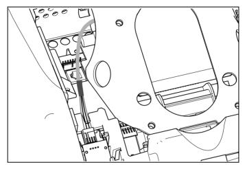
Figure 27: Connecting the heart rate cable
