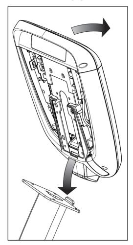
Figure 29: Console positioning on base unit
