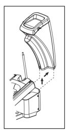
Figure 2: Lift cover removal
