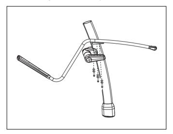
Figure 16: Upper body handlebar attachment detail
