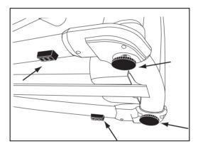
Figure 21: Rubber pad and adjustable foot locations
