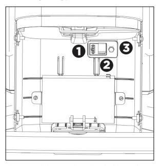
Figure 6: Cable connection points inside EFX base
