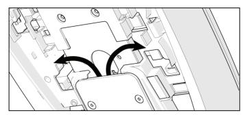
Figure 30: Cable routing from the mount into the console
