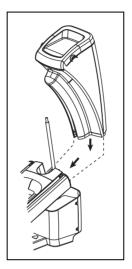
Figure 7: Lift cover replacement
