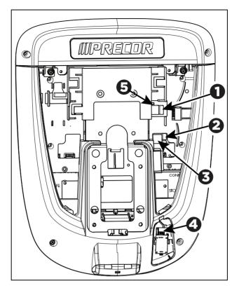
Figure 31: Cable connections, P30 and P10 consoles
