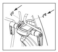
Figure 20: Axle cap attachment
