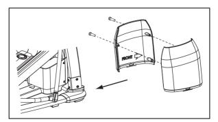
Figure 18: Upright support cover attachment (right-hand cover shown)
