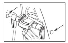
Figure 19: Pivot arm cap attachment
