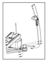
Figure 4: Attach the upright support to the base frame
