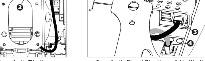
Connecting the Ethernet (3) and base unit data (4) cables
