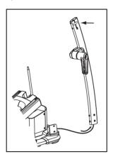
Figure 3: Thread cable through upright support
